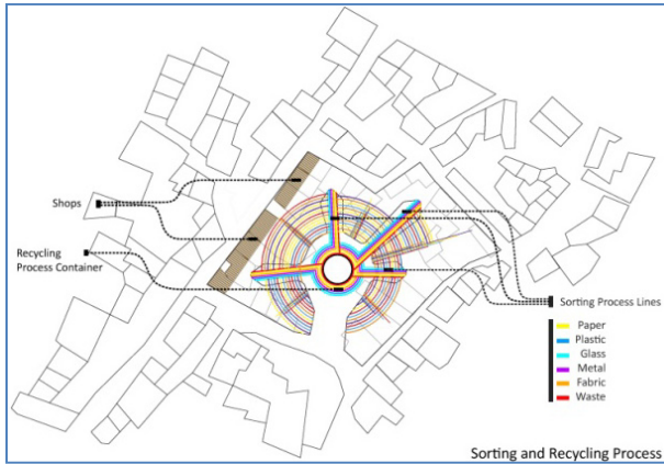
Figure 3: Sorting and Recycling Process. (Albadawy et al.)
