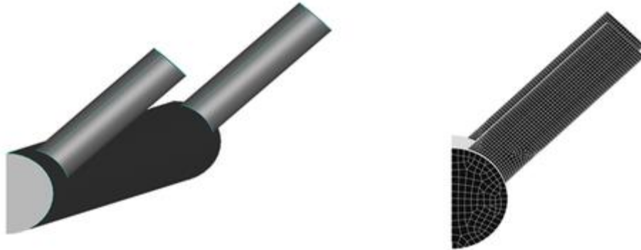
Computational domain *.stl file (left) and output mesh prepared in SALOME Meca (right)
