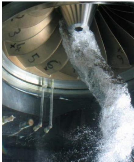
*Figure 1: Cavitating vortex rope in the draft tube of a Francis turbine (Seidel et al. (2014). Dynamic loads in Francis runners and their impact on fatigue life. IOP conference series: earth and environmental science, 22(3), 032054)*
