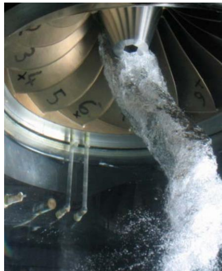
Abbildung 1: Kavitierender Wirbelzopf im Saugrohr einer Francis-Turbine (Seidel et al. (2014). Dynamic loads in Francis runners and their impact on fatigue life. IOP conference series: earth and environmental science , 22(3), 032054)
