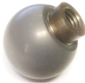
Fig. 8 Alumina ceramic head with titanium sleeve brazed
