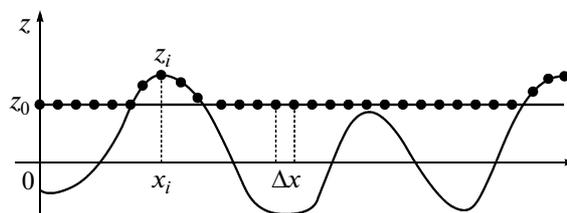
**Fig. 1.** One-dimensional model used in the method of dimensionality reduction for simulating the contact between an elastomer and a rough solid surface (see text for explanations).
