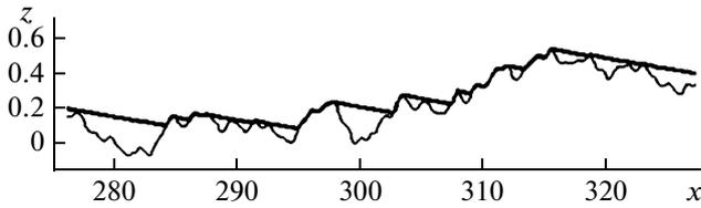
Fig. 2. "Snapshot" of rough solid surface—elastomer contact (thick solid curve) configuration.
