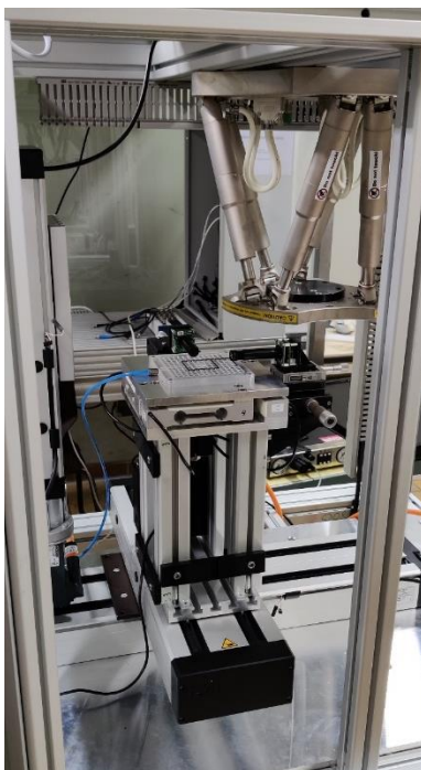
Figure 2: Interior of the machine with hexapod and linear axes
