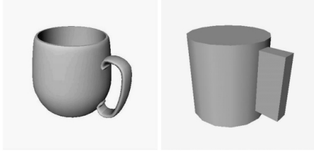
Figure 2.4: A coffee mug approximated by two shape primitives: A cylinder and a box. Image taken from [21].
