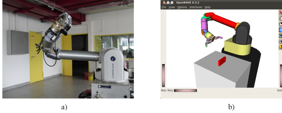
Figure 3.2: a) The eye-in-hand setup: Barrett Hand equipped with a camera around its wrist. b) The robot for experiments: WAM 7-DOF Arm with attached Barrett Hand, shown in the OpenRAVE simulator.
