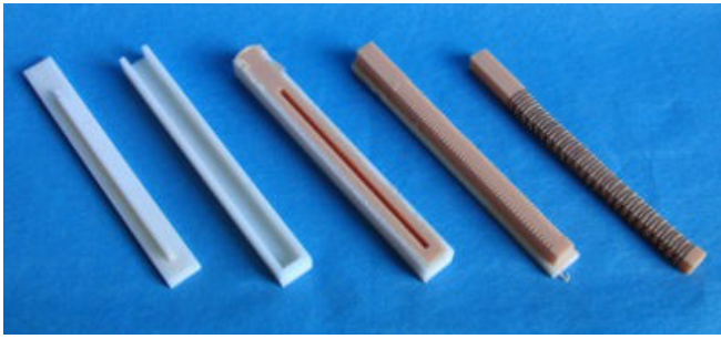
Fig. 5: Two-part mold, casts, and complete active layer with reinforcement helix
