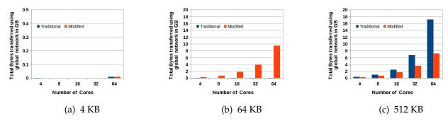
Figure 2: Total number of bytes (in Gigabyte) transferred by on-chip global network in our proposed cache protocol compared to a system using the traditional MOESI directory-based baseline protocol.
