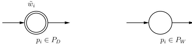
Figure 3.4: Graphical representation of places with holding times (left) and places without holding times (right)
