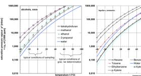
Figure 1: Saturation pressure of typical solvents for liquid sampling
