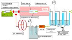
Figure 3: Test gas generator concept used, right test object
