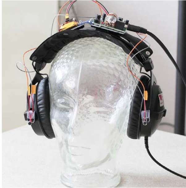
Figure 4.1.: The hear-through headset realised as closed-back circum-aural headphone with two microphones mounted on the enclosure.
