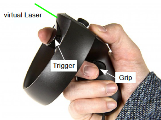
Fig. 10: Handheld Oculus Touch controller with grip and trigger button held.
