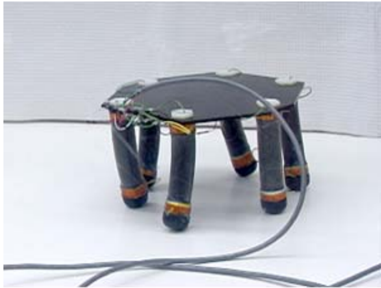
Figure 1.7: Hexapod robot MERbot using six spring roll actuators [37].
