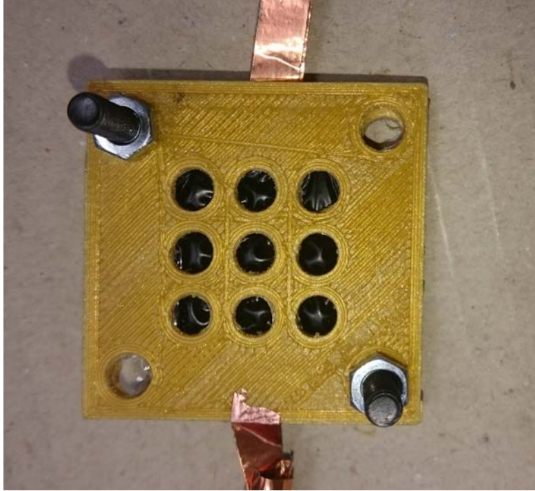
Figure 3.1: Experimental buckling DEA with membrane thickness of 50\text{ }\mu\text{m} with 3\text{ kV} supplied voltage. One large electrode was expected to buckle-up through the 5\text{ mm} wide cavities. The deformation could not be assumed as spherical.
