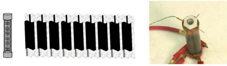
Figure 1.6: Schematic view of one spring roll actuator. Left: Spring; Middle: electrode pattern; Right: Actuator. [37]
